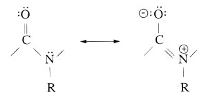
Figure 11. Resonance structures for a PHIC monomer unit.
